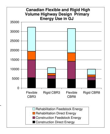
The feedstock energy component was the largest contributor to total energy for all of the asphalt pavement structures. Even when feedstock energy was excluded, Portland cement based concrete still enjoyed a significant energy advantage relative to its asphalt counterpart.
