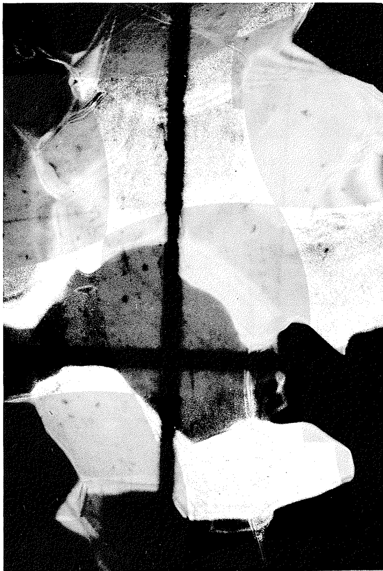
ENLARGED VIEW OF HORIZONTAL SECTION OF ICE LENS (MAG. 10 \times ) Heat flow normal to plane of photograph. Note irregular grain boundaries and uneven grain sizes.
