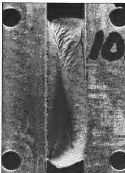
Figure 9 (left). Stage 2 of permanent deformation (exposure past one winter); south exposure, underside at preparation, \pm 65\% .
