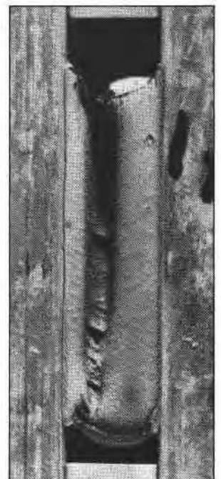
Figures 16a (left) and 16b (right). Three-year exposure on strain-cycling rack at \pm 30\% maximum yearly movement. 16a: south exposure, top at preparation; 16b: north exposure, underside at preparation.
