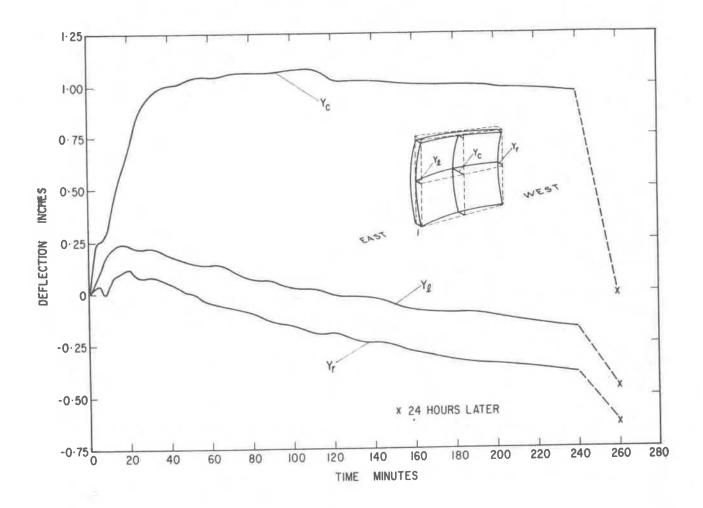
FIGURE 8 LATERAL DEFLECTION DURING FIRE TEST
