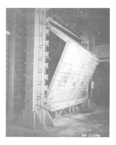
Figure 11 Collapse of the specimen during reload test
