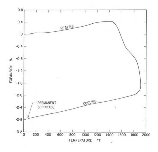
FIGURE 3 DILATOMETRIC CURVE HEATING RATE: 9 °F/MIN
