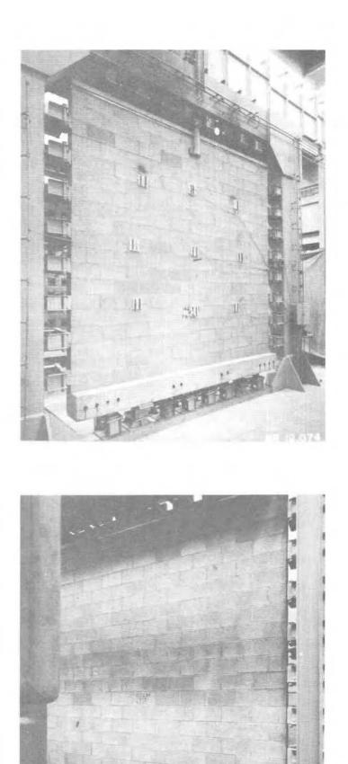
Figure 4 Reverse side of the specimen prior to fire test
