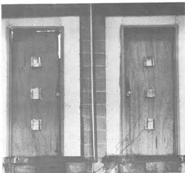
Figure A61. Door Test No. 10. Unexposed face following fire exposure and hose stream.
