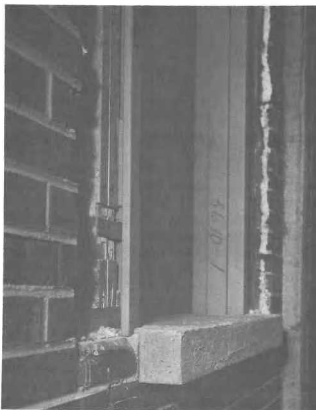
Figure A17. Door Test No. 2. Installation of steel frame.
