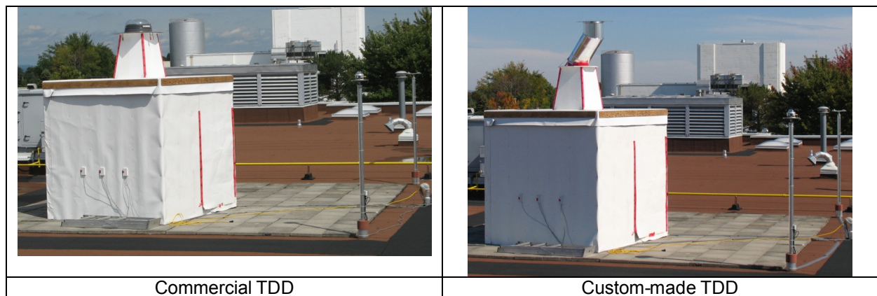
Figure 8 Geometrical details of the custom-made TDD product C with an elbowed pipe (tilted middle section and vertical upper and lower sections)
