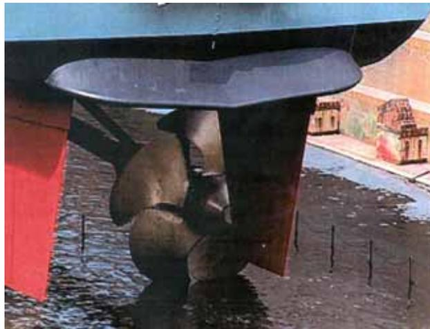
**Figure 11: Stern Flap Installed on the USS Curtus Wilbur (DDG 54)**
