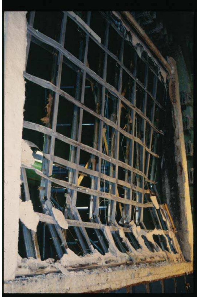
Figure 4. Steel Stud Wall Assembly after Fire Resistance Test.
