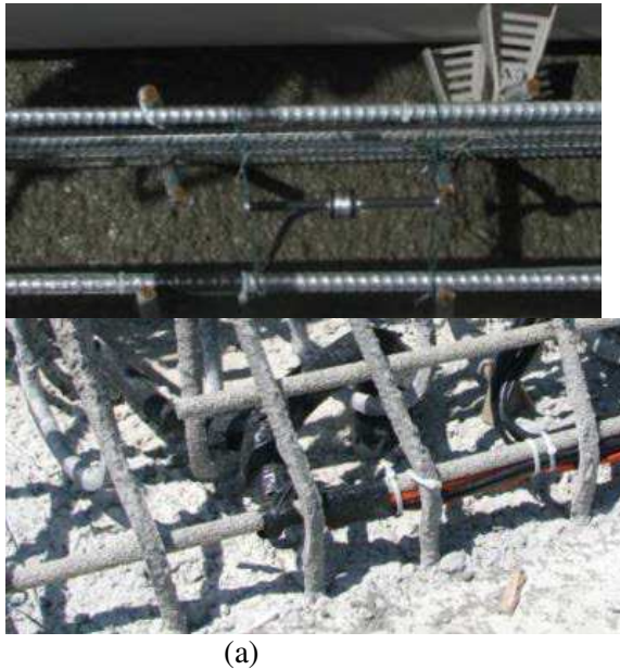
Figure 5. Instrumentation of the barrier: (a) VWSG (EM5) embedded in concrete; (b) Thermometers (TH-T) attached to the reinforcing bars
