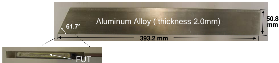
Figure 17. One FUT coated directly onto the top surface near the edge of an Al plate with an angle of 61.7^\circ to generate and receive SH PAW.
