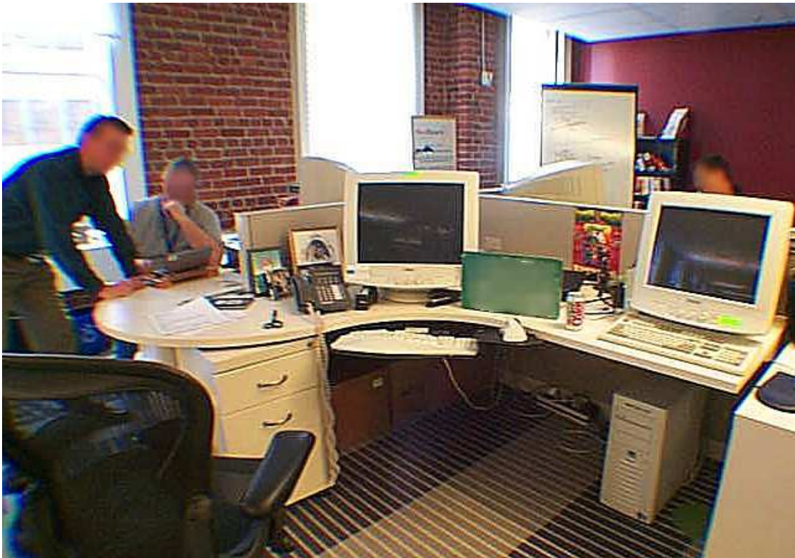
Figure 3. In this office, the low panels between workstations provide access to daylight and view for occupants in the interior. However, these low panels provide little acoustic or visual privacy.
