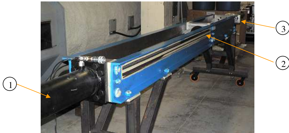
Fig.3) Experimental rig for tests: 1) cylinder for pulling the tube, 2) location of installation of die, 3) cylinder for movement of mandrel.
