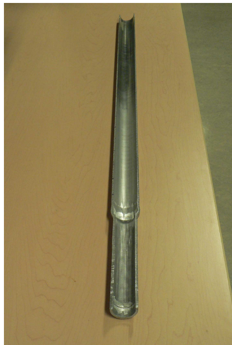
Fig.4) The tube produced using tube drawing machine of Laval University.
