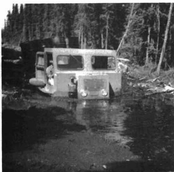
Figure 6 Scout Car with trailer successfully negotiating difficult muskeg conditions loaded with 4 tons of fuel.
