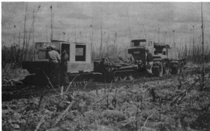
Figure 1 From left to right, a Weasel with a track trailer and a North King fitted with tracks. The North King proved to be too heavy for muskeg.
