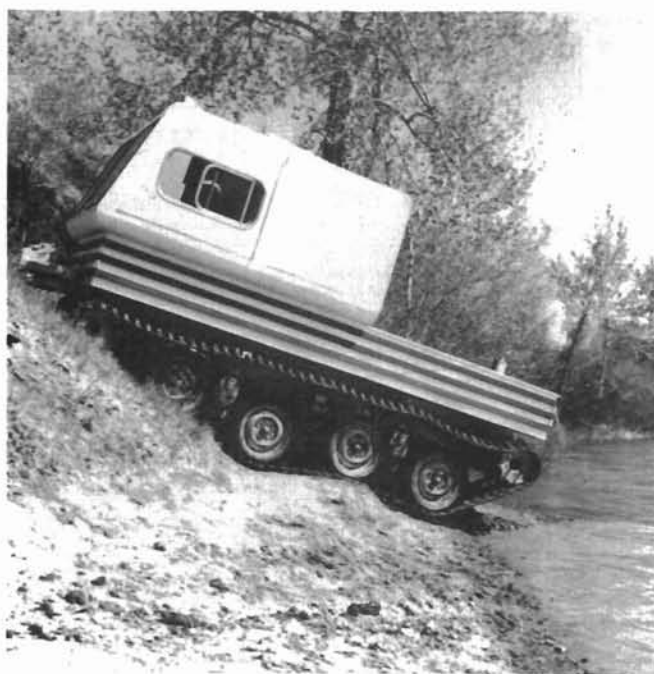
Figure 2 A hydraulic drive track vehicle built by Imperial Oil Limited. Its success was defeated by mechanical troubles.
