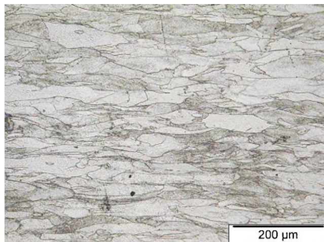
Fig. 2. Optical micrograph of ULC steel after 3000 s annealing. Deformation and annealing temperature = 550 °C, strain = 0.5, strain rate = 0.1 s −1 .
