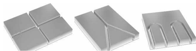
Fig. 7 Optical profilometry of embossed devices (Zeonor 1060R): cruciform structure (left), splitter (middle) and serpentine race (right), structure depth = 20 \mu\text{m} , channel width 50 \mu\text{m} .
